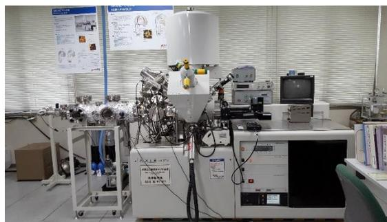
Fig. 13 X-ray photoelectron spectrometer (AXIS-Ultra DLD, Kratos)
