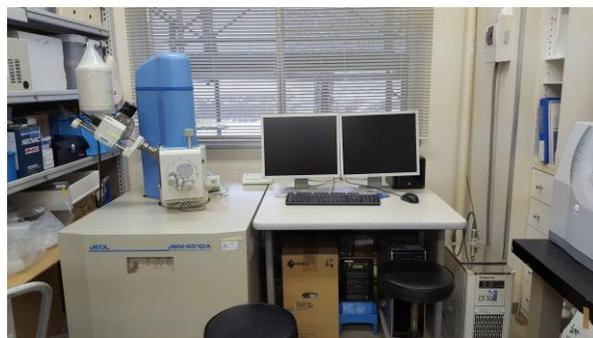
Fig. 4 Scanning electron microscope-Energy dispersive X-ray spectrometer (JSM-6520A, JEOL)
