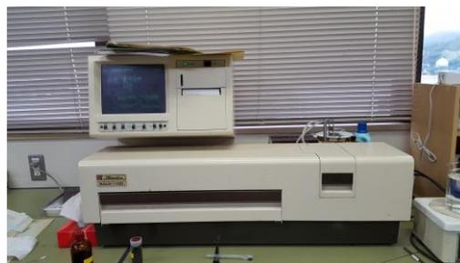
Fig. 2 Laser diffraction particle size analyzer (SALD-1100, SHIMADZU)
